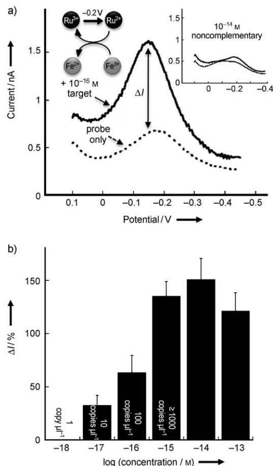
**Figure 2.** Electrochemical microRNA detection: readout and sensitivity. a) Differential pulse voltammetry (DPV) showing the signal increase observed after incubation of the complementary target (miR-21, 100 aM) with a probe-modified NME for 30 min. The signal observed with a noncomplementary target at a 100 times higher concentration is shown in the inset. b) Determination of the sensitivity and detection limit for electronic miR-21 detection.
