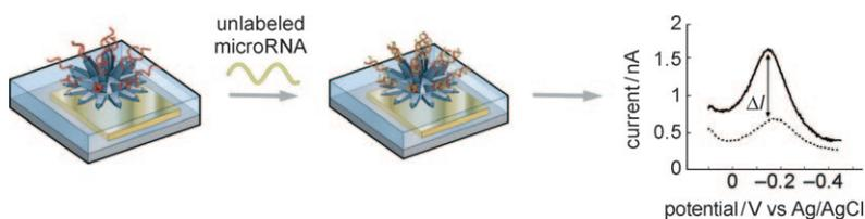
**In the time it takes for lunch:** An electronic chip featuring nanostructured microelectrodes (NMEs) enables the analysis of microRNA expression profiles in just 30 min in small RNA samples without enzymatic amplification or
